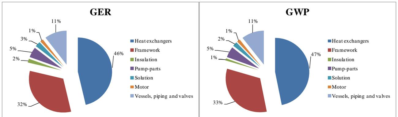
**Figure 4: Percentage contribution of different chiller components to GER and GWP**
