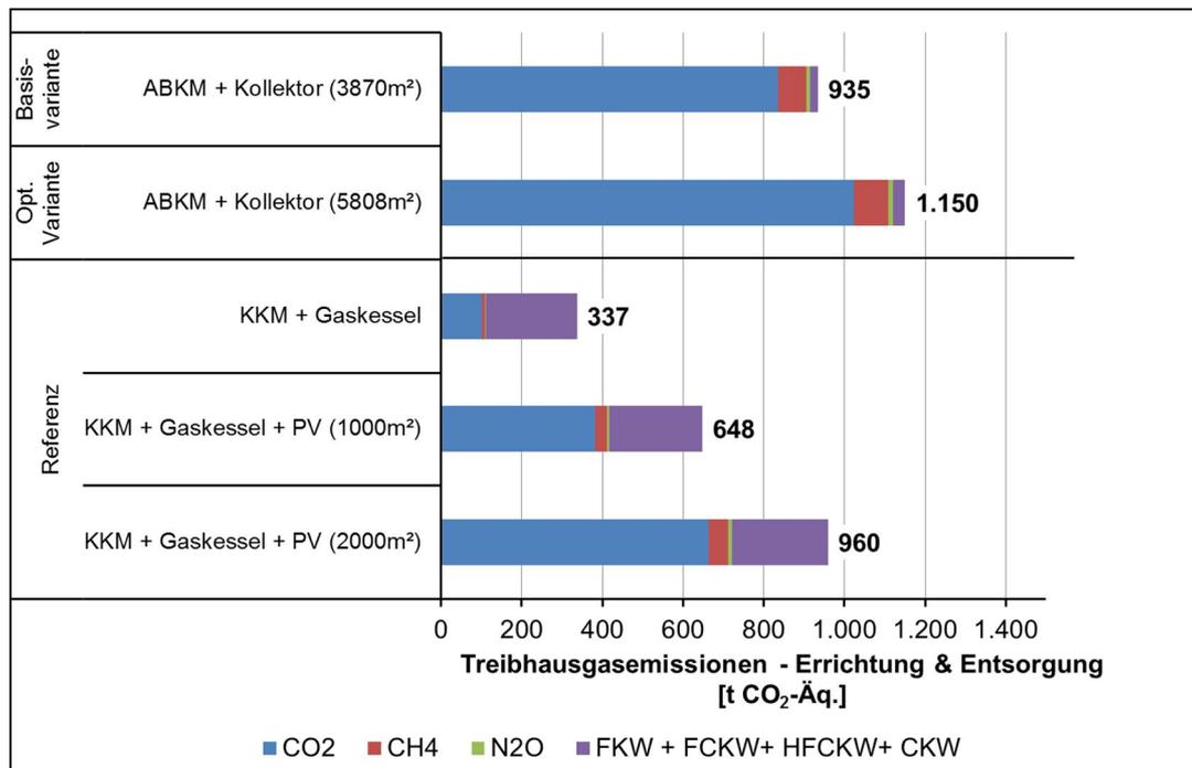
**Figure 11: Case study " Absorption chiller H<sub>2</sub>O-LiBr, refrigeration capacity 1470 kW": greenhouse gas emissions from construction and waste disposal for the base variant, the optimized version and the reference systems divided into the type of greenhouse gas emissions; refrigerant of the compression chiller: R410A**
