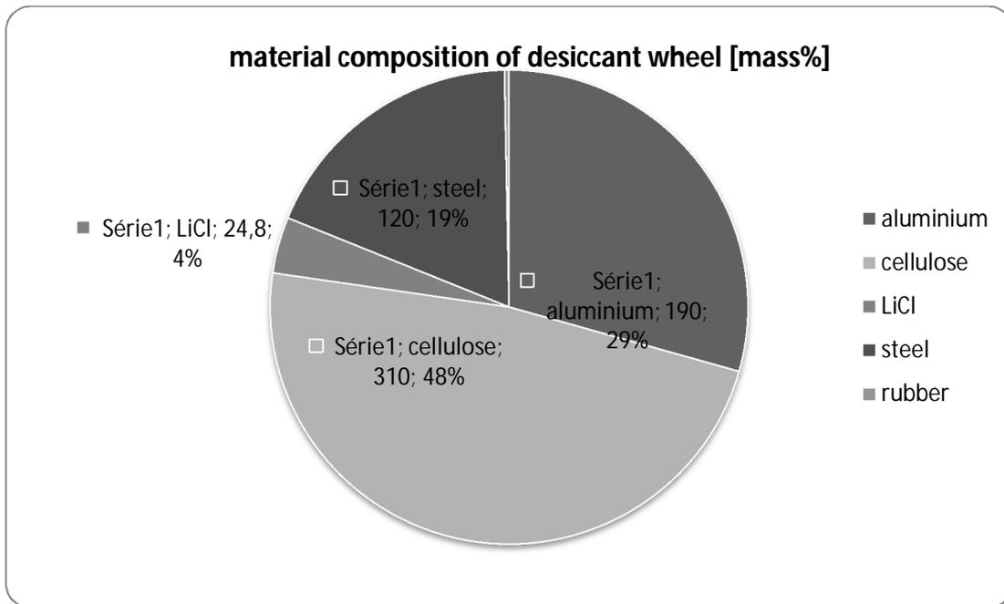
Figure 8: Material composition of desiccant wheel in a SDEC system (based on information from robatherm and Klingenburg)
