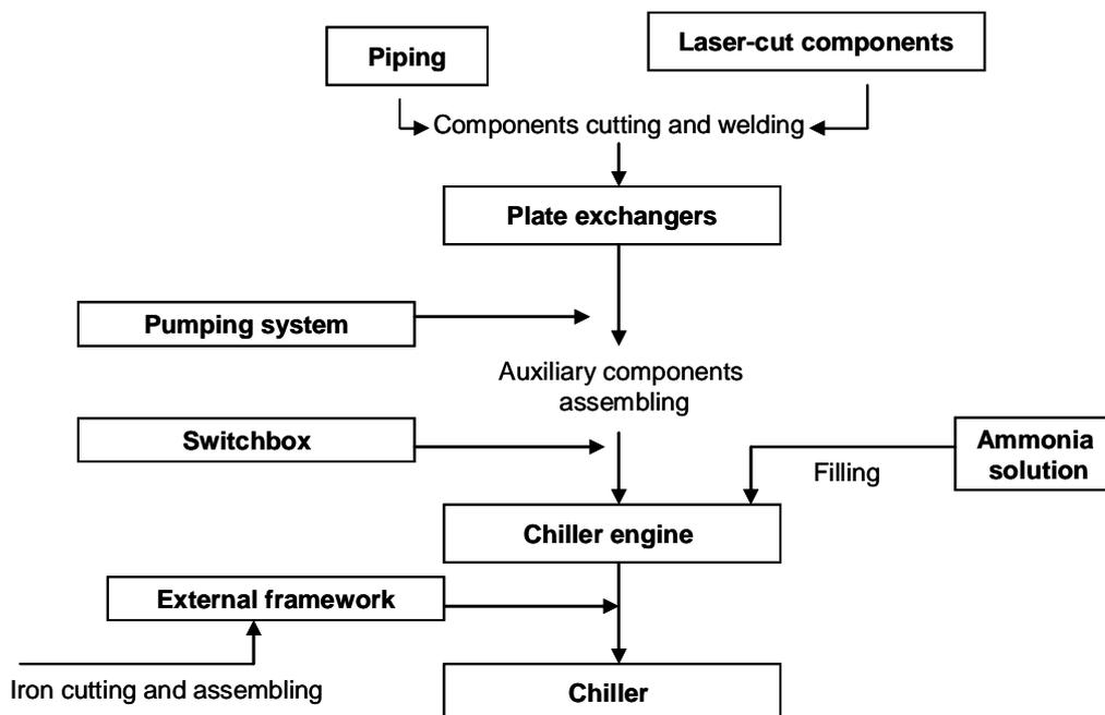
**Figure 2: Production diagram flow**
