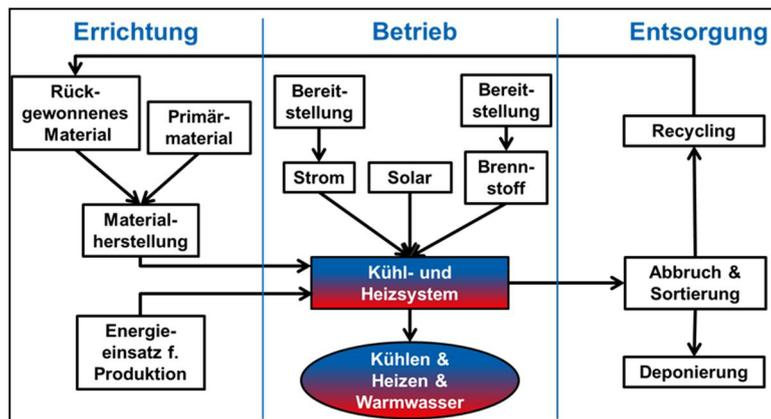
Figure 10: System boundaries in construction, operation and disposal
